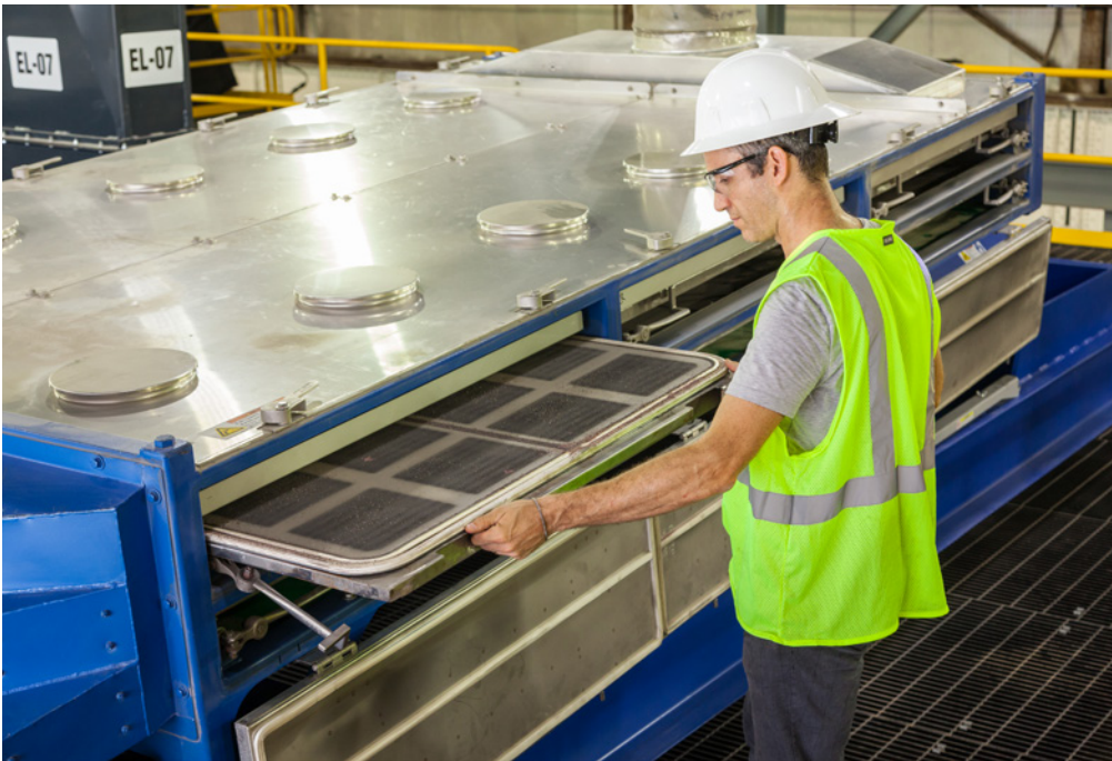
Segmented screen panels provide easy access for fast maintenance and higher productivity.
