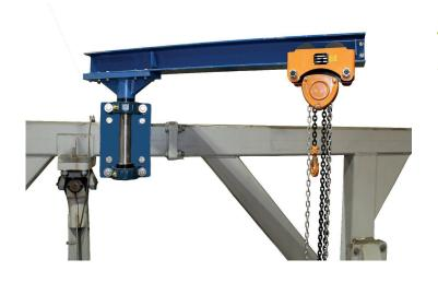
Hoist facilitates maintenance to lift drive weights, motors, and drive cartridges.
