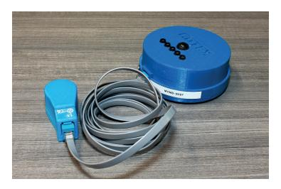
Allows you to measure structural vibrations for the dynamic analysis of support structures.
