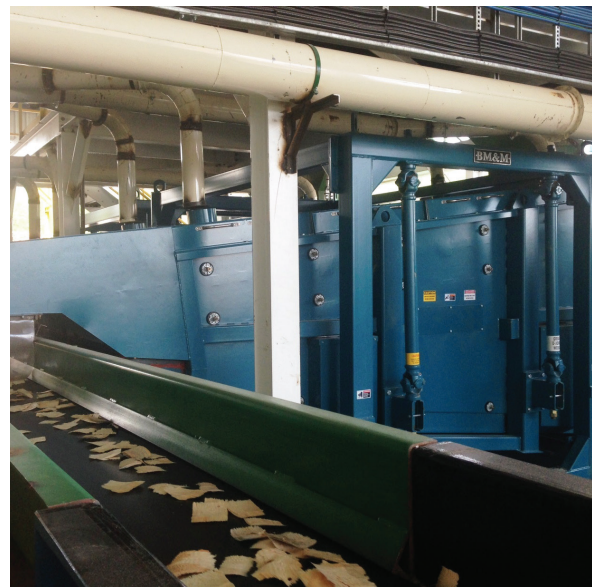
A modern BM&M Counterflow Chip Screen used in a wood chip screening application.
