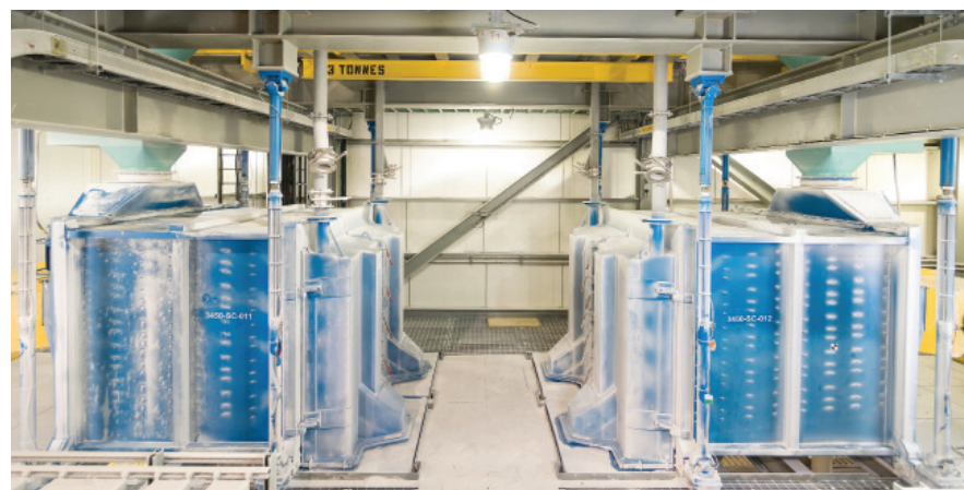
Figure 5: KSPC fertilizer product loadout area; two Rotex Model MM5430-2 mineral separators
