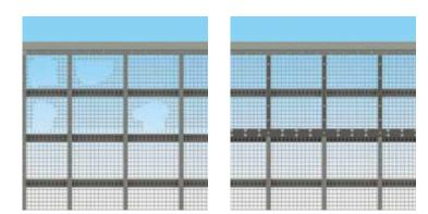
Extend the life of a worn screen frame by replacing only the tattered section of the ball support.
