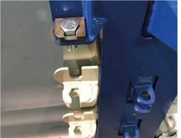
Drop-on flats hold the bolt head, reducing installation time and requiring only one wrench during screen replacement.
