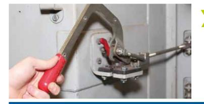
The locking trigger secures the door clamp during operation. Easy to follow instructions are provided for installing replacement triggers. New clamp assemblies are also available.
