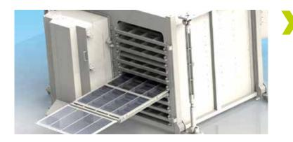
Reduce time and effort for screen maintenance. Screen panels do not require tensioning andcan be replaced without the need to removescreen frames from the machine. These also provide the option for different mesh sizes in a single deck..
