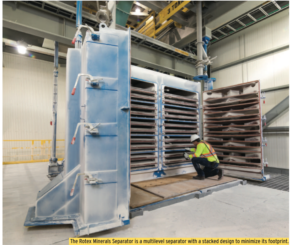
The Rotex Minerals Separator is a multilevel separator with a stacked design to minimize its footprint.
