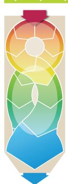
The Gyratory-Reciprocating Motion gradually changes along the length of the machine to an elliptical path and finally to an approximate straight line motion at the discharge end.
